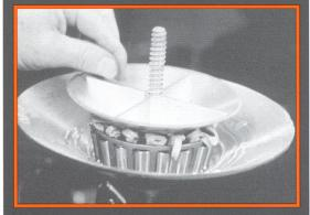
Any excess grease should be smeared on the outside of the rollers.
